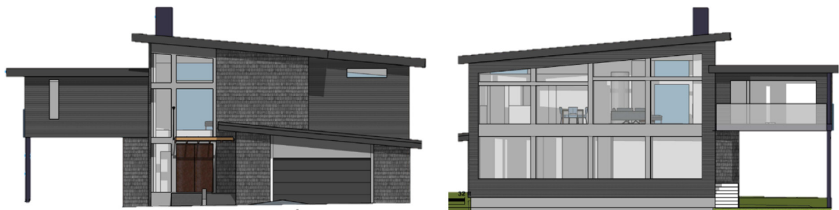
Fig. 6. A sample house designed to Step 5 of the Energy Step Code. Left: South Elevation, right: North Elevation.
