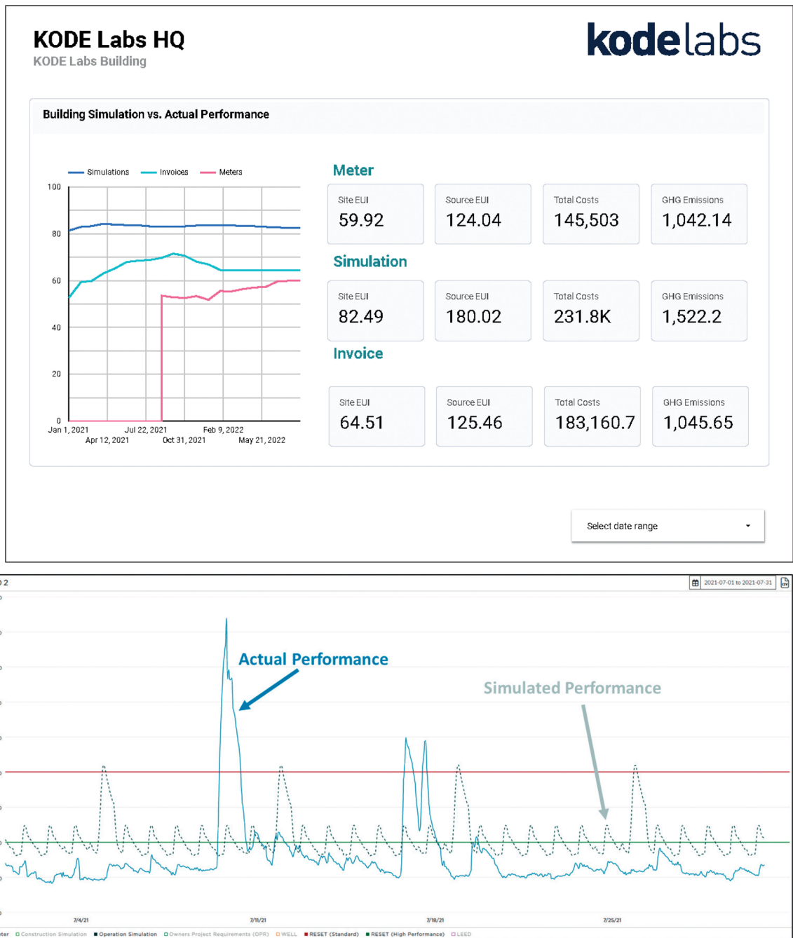
Figure 5 Integrating building science and data science
